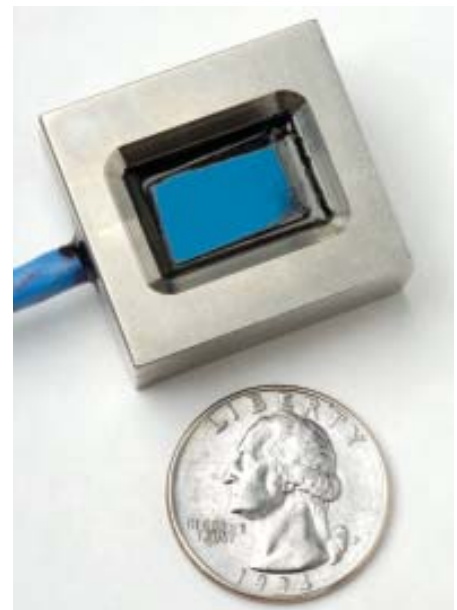
Figure 2. Commercially available solid-state viscosity sensor.
