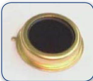
Figure 7: ViSmart™ sensor element at the start of the RPVOT test
