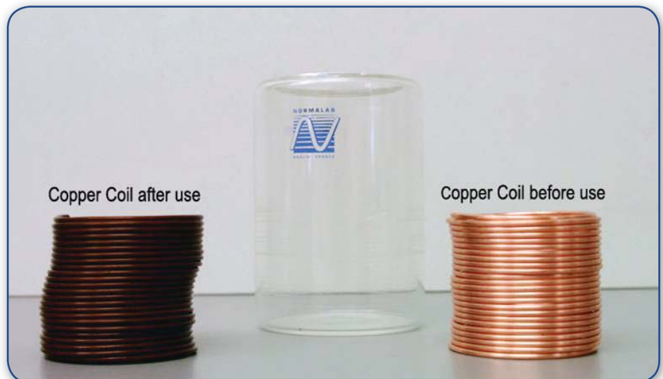
Figure 4: The effect of RPVOT testing on the copper coils
